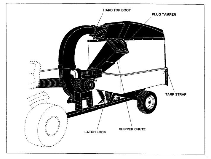
HARD TOP BOOT Connects the plastic elbow to the hard top, directing discharged material into the cart.
